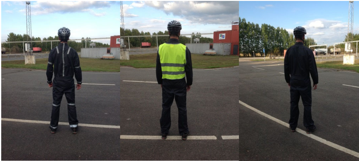
Fig. 1. Reflective clothing patterns from left to right: biomotion, vest and legal minimum.
